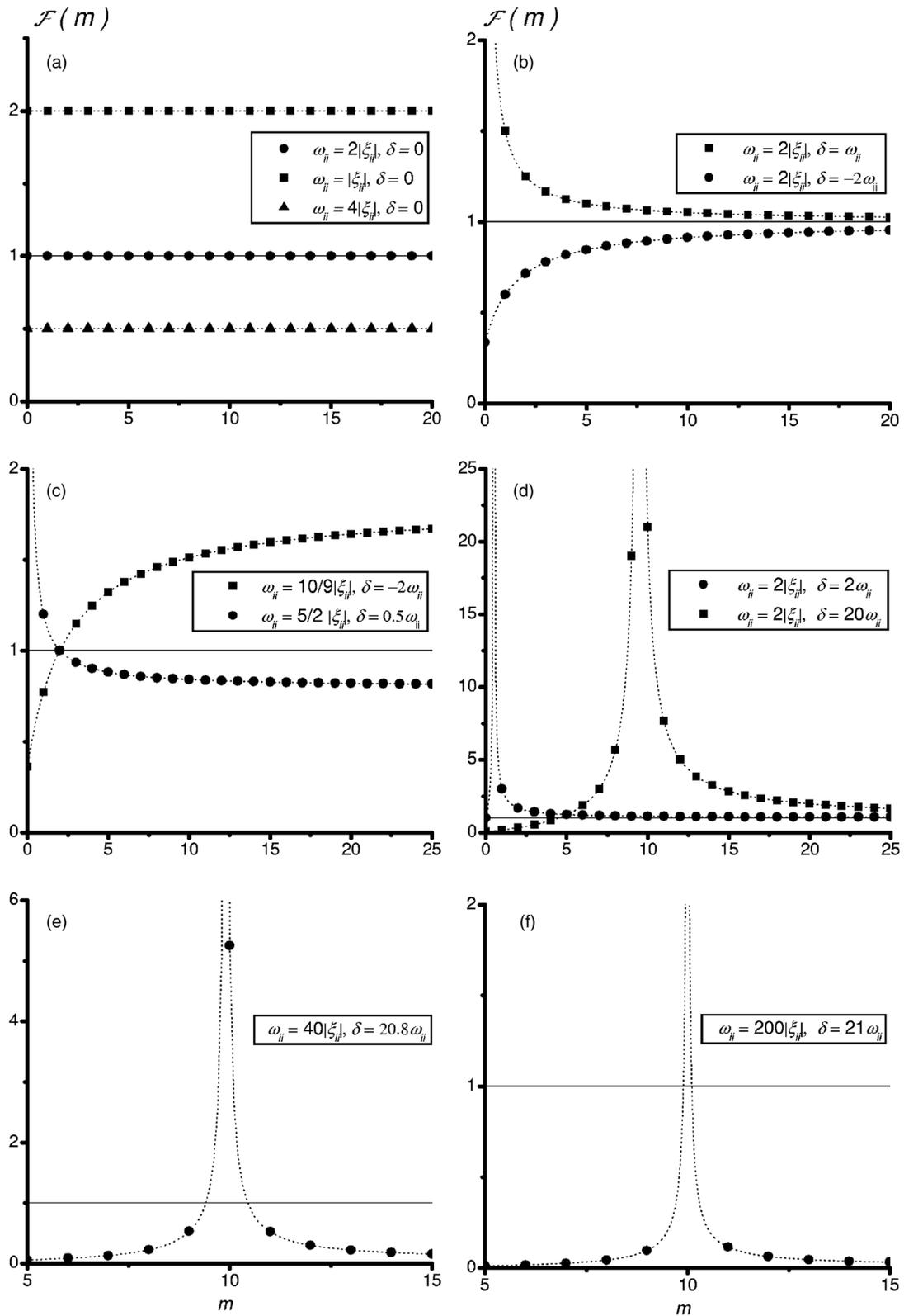
FIG. 2. Distinct forms of behavior of  $\mathcal{F}(m)$ , for different values of  $\omega_{ii}$  and  $\delta$ , which determines the regimes of the parametric amplification processes.
