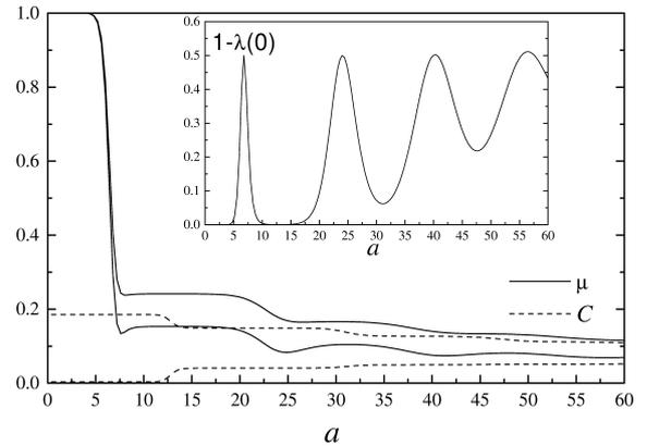
Fig. 6. The “purity”  $\mu$  and the “coherence”  $C$  versus  $a = |\alpha_0|^2$  for the initial circular states with  $N = 16$  and  $\nu = 0$ , for two different values of “compact time”  $u$ . Solid lines are for  $\mu$  and dashed lines are for  $C$ . Upper curves correspond to  $u = 0.1$ , lower curves are for  $u = 0.3$ . In the insertion: the difference  $1 - \lambda(0)$  versus  $a$ .
