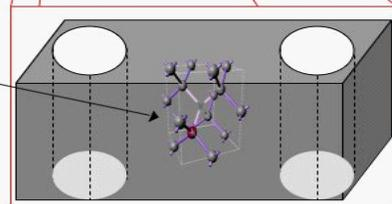
**Nitrogen-Vacancy center (or any 2-level dipole-coupled system)**
