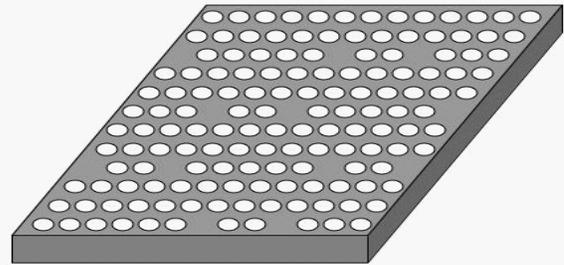
**Step 3:** Implant nitrogen atoms in each defect to create NV centers in each PBG defect optical cavity. Now we have an interconnected array of cavity-QED sites.
