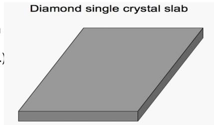
**Imaginary Step 2:** Create a photonic band gap material by drilling holes periodically in your slab with the lattice spacing  $a$  given by the wavelength of light you want to use.
