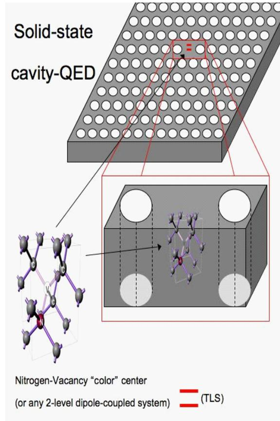
**Step 2:** Make the defect cavity super-lattice for real by drilling holes on a lattice everywhere except where we want the cavities to be. We make the defect cavities close enough such that there can be a possibility of photon hopping between nearest neighbors.
